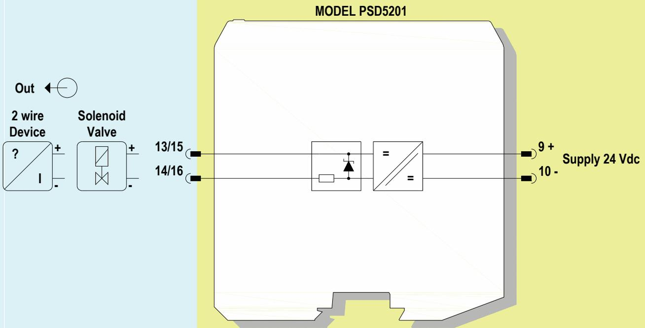
Application of PSD5201 for NE load
